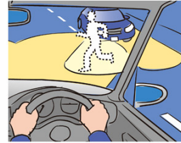
Due to the evaporation phenomenon, the driver might lose sight of a pedestrian.
